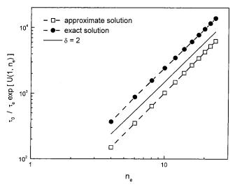
**Figure 4.** Preexponential dependence of the terminal relaxation time  $\tau_0$  on the number of entanglements per star arm,  $n_{\rm e}$ . The exponential dependence of  $\tau_0$  on  $n_{\rm e}$  has been normalized out to more clearly reveal the form of the preexponential factor. Key: open squares, approximate solution; filled circles, exact solution. Solid line, shown for comparison, corresponds to a power-law exponent  $\delta=2$ .
