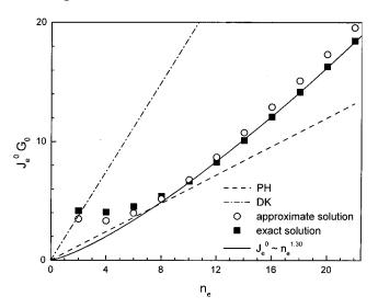
**Figure 8.**  $J_e{}^0G_0$  vs the number of entanglements per star arm  $n_e$ , calculated from both the approximate (open circles) and exact (filled squares) solutions to the MM theory. Lines shown for comparison represent  $\phi = ^{15}/_8$  (DK theory, dot—dashed line), 0.6 (PH theory, dashed line), and a power-law dependence with exponent  $\kappa = 1.30$  (best-fit to the exact MM results for  $10 \le n_e \le 24$ , solid line).
