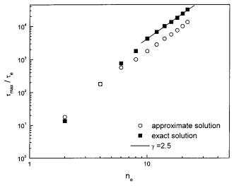
**Figure 6.** Reciprocal of the frequency at the peak of  $G''(\omega)$ , denoted as  $\tau_{\text{max}}$ , vs  $n_{\text{e}}$  as predicted by the MM model (filled squares, exact solution; open circles, approximate solution).  $\tau_{max}$  is normalized by the basic microscopic time  $\tau_{e}$  (Rouse time of an entanglement segment). The solid line is a power-law fit to the data at high  $n_e$ , with an exponent  $\gamma = 2.5$ .
