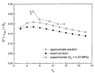
**Figure 7.** Magnitude of  $G''(\omega_{\text{max}})$  as a function of  $n_{\text{e}}$  as predicted by the model (filled squares: exact solution; open circles: approximate solution).  $\hat{G}'(\omega_{\max})$  is normalized by the plateau modulus  $G_0$ . Open diamonds: data of Graessley and Roovers<sup>23</sup> for 4- and 6-arm star polystyrenes, normalized by  $G_0 = 0.20 \text{ MPa}.$
