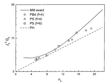
**Figure 9.** Experimental values of  $J_e{}^0G_0$  vs the number of entanglements per star arm  $n_e$ . Key: diamonds, four-arm polybutadiene stars;<sup>22</sup> triangles, four-arm polystyrene stars;<sup>23</sup> squares, six-arm polystyrene stars.<sup>23</sup> Predictions of the PH theory (dashed line) and MM theory (exact solution, solid line) are shown for comparison.  $G_0$  values employed<sup>24</sup> were 1.15 MPa for polybutadiene and 0.20 MPa for polystyrene.
