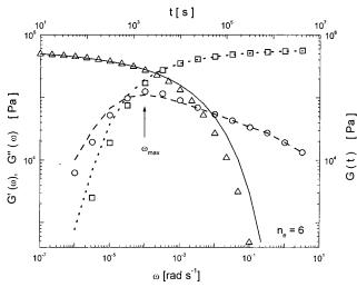
Figure 5. Linear viscoelastic moduli predicted by the approximate solution (symbols) and exact solution (lines) to the MM theory. Results calculated with representative parameters,  $n_{\rm e}=6$ ,  $G_0=0.6$  MPa,  $\tau_{\rm e}=15$  s. Left axis: squares and dotted line,  $G'(\omega)$ ; circles and dashed line,  $G'(\omega)$ . Right axis: triangles and solid line, G(t).
