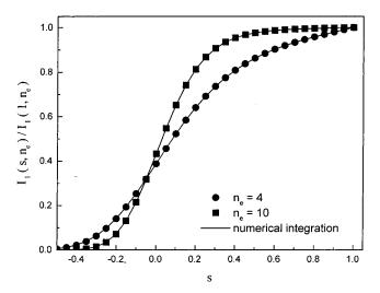
Figure 1. Exact solution to the inner integral in the firstpassage time (FPT) problem,  $I_1(s, n_e)$ , normalized by the value at s = 1 (complete retraction), for  $n_e = 4$  (circles, 10 terms in series) and  $n_e = 10$  (squares, 20 terms in series). Numerical evaluations of the same integrals are shown as the continuous curves.
